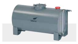
**Spraying tank** made of stainless steel, capacity 69 l, filter insert (stainless steel), with level indicator, drainage aperture and quick-release coupling for the connection of the chemical feed line.
