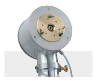
**Spraying head** of the Fontan Mobilstar with adjusting disc for ULV and LV. In the "LV" position, the air volume at the nozzle is reduced, thus producing larger droplets.
